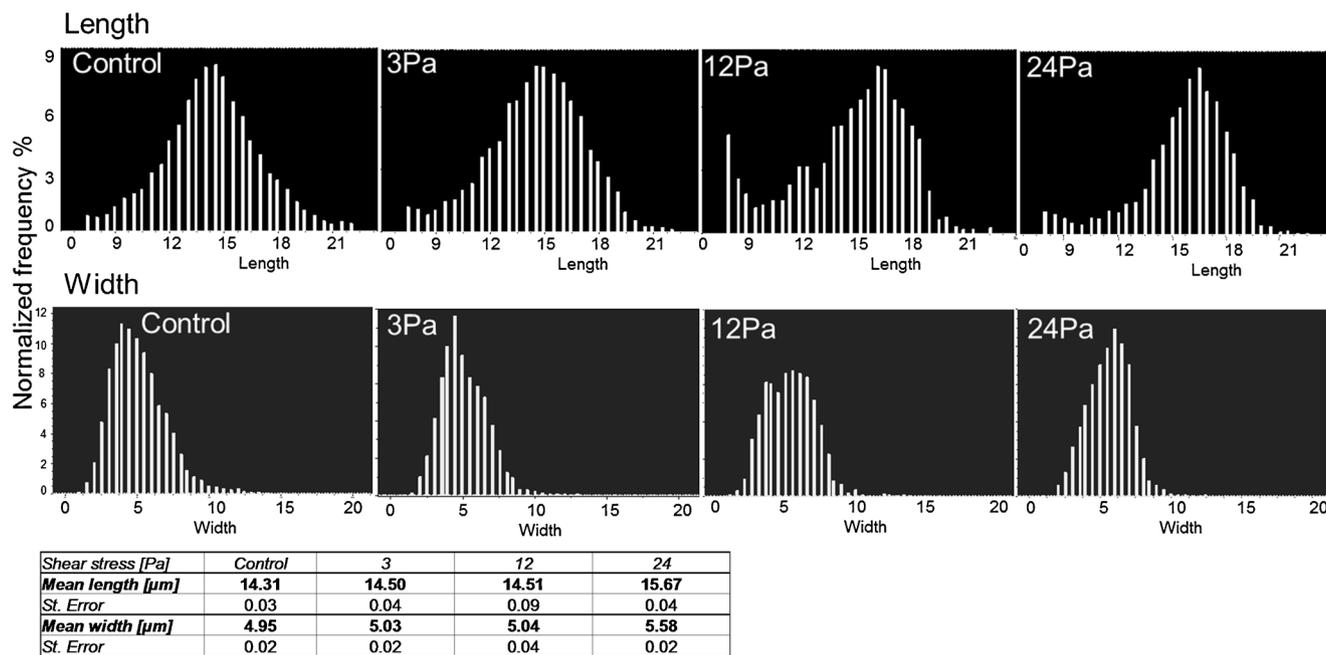
**Fig. 7** Differences in length (*upper panels*) and width (*lower panels*) of *A. coffeaeformis* silica particles in the control sample and the eluent collected from the slide exposed to increasing shear force (3–24 Pa)
