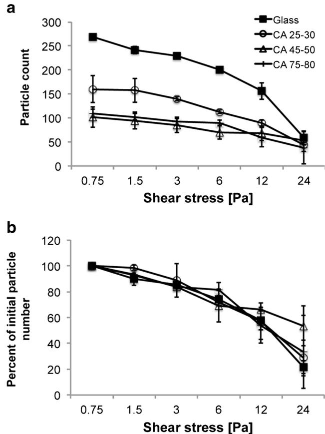
**Fig. 4** Adhesion of *A. coffeaeformis* silica particles on substrates of varying hydrophobicity after incremental increases in shear stress shown as: **a** number of particles remaining on the slide after each pressure applied; **b** percentage of initially adhered particles. CA - contact angle. The data are mean  $\pm$  SE of three independent experiments
