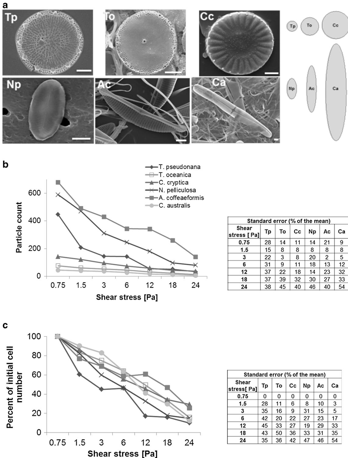
**Fig. 5 a** SEM images of silica valve structures from diatom species chosen for comparison of adhesive properties, and a schematic of their relative size and geometric representation. Centric diatoms: Tp- *Thalassiosira pseudonana*; To- *Thalassiosira oceanica*; Cc- *Cyclotella cryptica*. Pennate diatoms: Np- *Navicula pelliculosa*; Ac- *Amphora coffeaeformis*; Ca- *Craspedostauros australis*. The scale bar is 2  $\mu\text{m}$ .
